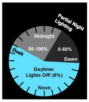
conditions. Motion sensors can be added to these controls to turn lights back on when movement is detected. Dimming, Dimming or bi-level switching reduces lighting levels when bi-level switching, or curfew lighting controls can also combination of controls can work very well for parking lots.
